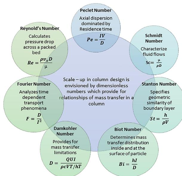
Fig. 3. Significance of dimensionless numbers in Scale-up/Scale-down.
