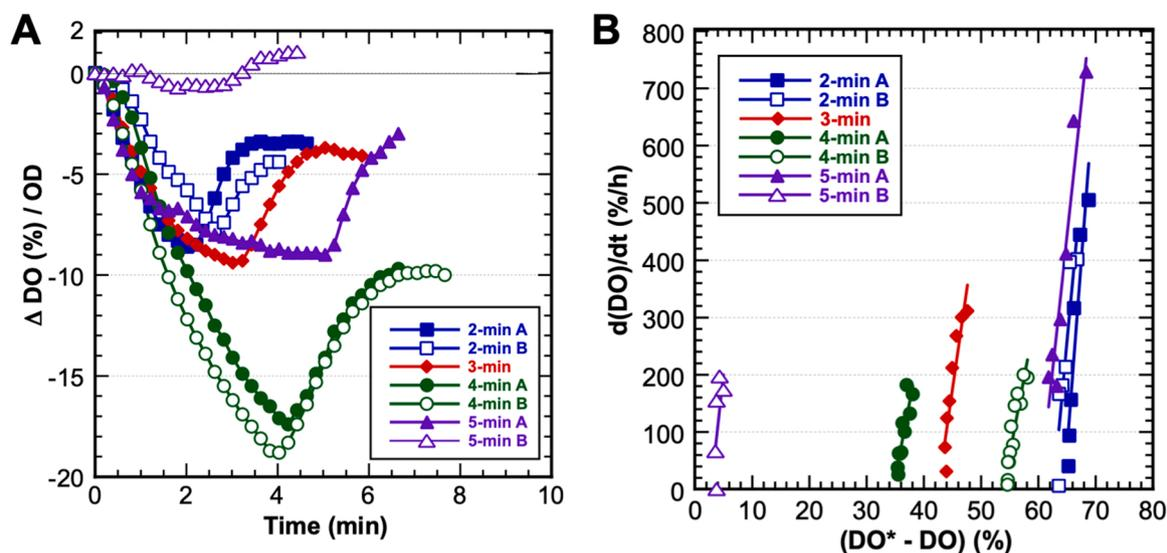
Fig. 3. The  $k_La$  estimates using the minimally-disruptive method for *E. coli* pTV1GFP in the ambr250 modular bioreactor. A) Reaeration curves, where the change in DO was normalized to the OD at the beginning of the test; B)  $k_La$  estimates were obtained from the slope of the difference between DO and  $DO^*$  versus the time derivative of the DO change. Replicate event durations are indicated by A and B.
