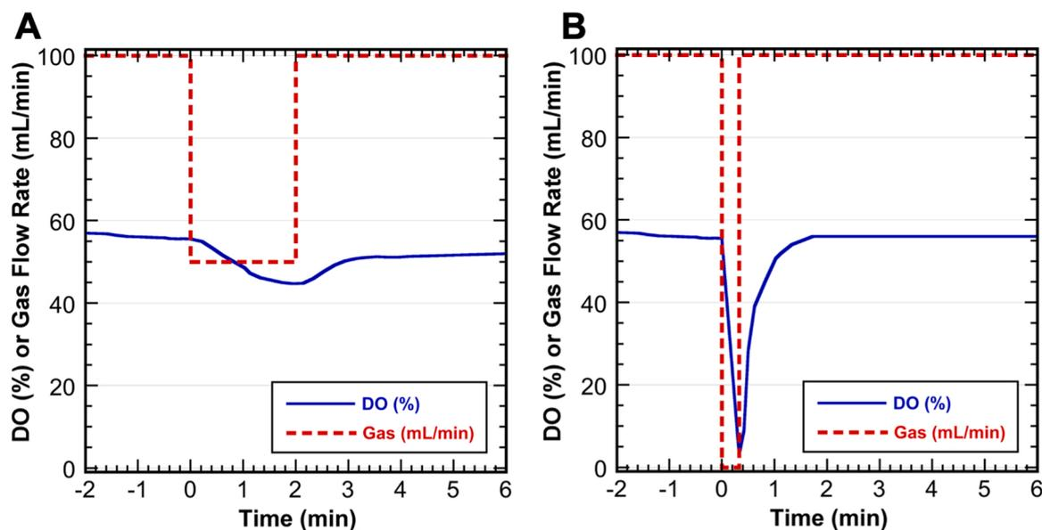
Fig. 1. Comparison of DO and gas rate flow profiles for the minimally-disruptive method and the dynamic gas-out method. A) Minimally-disruptive method, B) Dynamic or disruptive method. The DO (% saturation) profiles are shown as solid lines. The gas flow rate (mL/min) profiles are shown as dashed lines. DO and gas flow rates profiles in B) adapted from Tribe et al. [37].
