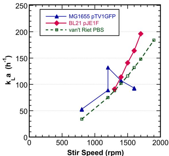
**Fig. 6.** Minimally-disruptive  $k_La$  estimator method used for two *E. coli* strains in ambr250 modular bioreactors. The  $k_La$  estimates versus stir speed for *E. coli* MG1655 pTV1GFP (variable duration, blue triangles ▲), *E. coli* BL21 pJE1F (2-min duration, red diamonds ◆), and extrapolation of the van't Riet equation fit of ambr250 bioreactor data obtained for 1.0 and 1.5 vvm ranging from 1900 to 4200 rpm stir speeds; data provided by manufacturer (green, unfilled squares ■).
