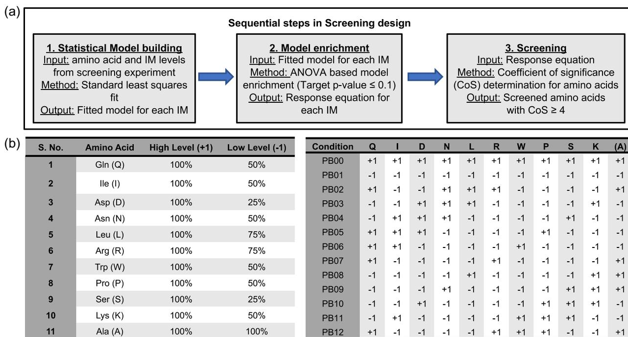
**FIGURE 4** (a) Sequential steps constructed in screening design to reduce the precursor design space. (b) Screening design matrix with different amino acids. Thirteen conditions were tested with various combinations of 11 amino acids at high (+1) and low (-1) levels.
