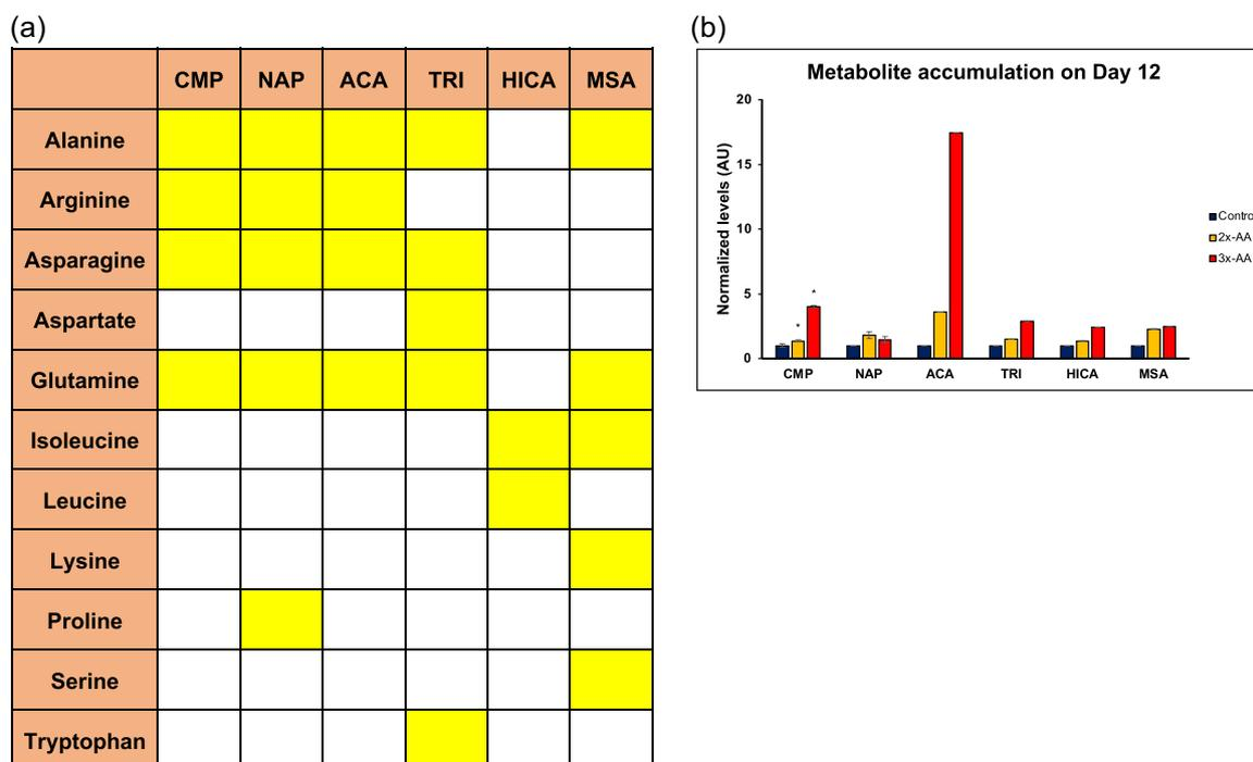
**FIGURE 3** Design and results of experimental pathway analysis for lumped source identification of metabolites in fed-batch cultures. (a) Amino acid substrate precursor matrix for each inhibitory metabolite and (b) inhibitory metabolite levels in cell culture supernatants on day 12 of fed-batch cultures. Mean  $\pm$  SD;  $n = 2$ ,  $*p < 0.1$ . Statistics by unpaired two-tailed student  $t$  test against control.
